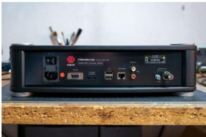
For the digital output, Avik relies exclusively on SPDIF. A BNC and a Toslink connection are available for this. For external storage media, there are 2 USB ports and, of course, an Ethernet port. Obviously, nothing works without Ethernet!
