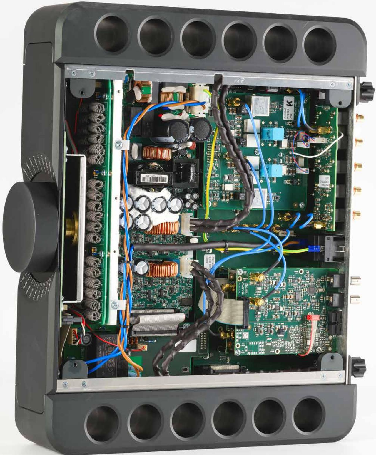
Free oscillation allowed here, damping with adhesive achieved there: Aavik's magic machine has resonances firmly under control like no other amplifier. All cables, including those of the 36 oscillating circuits on the left, are assembled and fitted by hand by the Danes in a process lasting dozens of hours.
