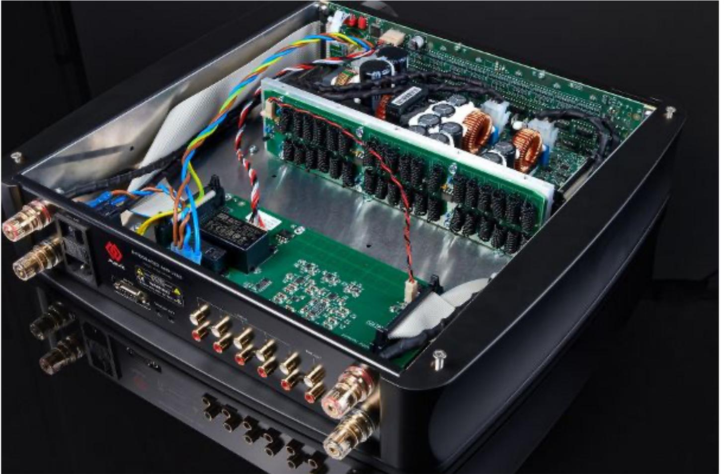
The high-quality and specially designed interior of the I-180: Well visible is the battery of the handmade voice coils (upright, centered).
